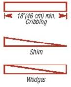
free of any paint or finish because this can make the wood slippery, especially when it is wet. Cribbing can be made out of pieces of timber found in the debris and cut to size. Pieces of 2X2 (5 cm X 5 cm) and 4X4 (10 cm X 10 cm) as well as wedges cut in this size timber are very useful.
