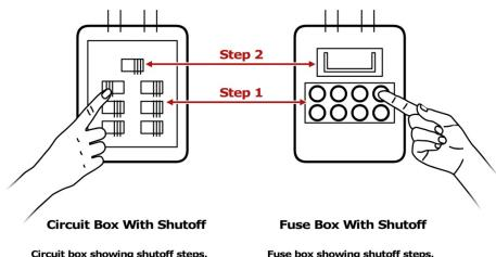
Circuit box showing shutoff steps. Step 1: Shut off individual breakers. Step 2: Shut off main breaker. Fuse box showing shutoff steps. Step 1: Pull out individual fuses. Step 2: Pull out main fuse.
