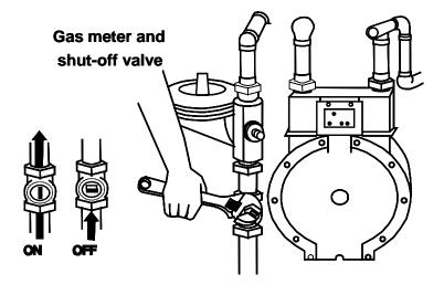
Please note: Some gas meters have automatic shutoff valves that restrict the flow of gas during an earthquake or other emergency. These are installed by a licensed plumber, downstream of the utility point of delivery. If you are unsure whether your home has this shutoff device, contact your gas service company. If this shutoff device is closed, only a qualified professional should restore it.
