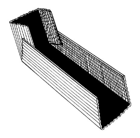
Cardboard Splint in which the edges of the cardboard are turned up to form a "mold" in which the injured limb can rest.
