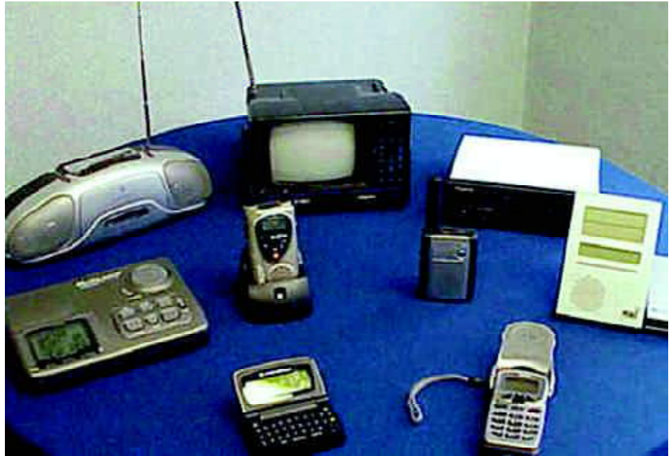
Electronic equipment available to receive weather information/NOAA (Weather Radio, Radio, TV, Pager, Cell Phone, Two-Way Radio)
