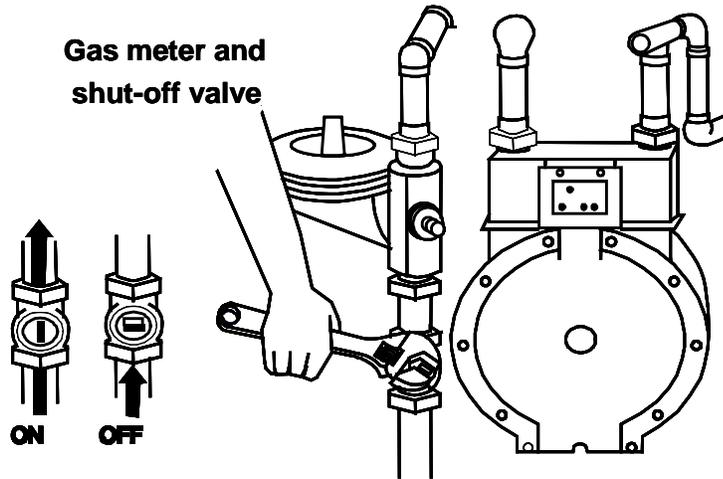
**Please note: Some gas meters have automatic shutoff valves that restrict the flow of gas during an earthquake or other emergency. These are installed by a licensed plumber, downstream of the utility point of delivery. If you are unsure whether your home has this shutoff device, contact your gas service company. If this shutoff device is closed, only a qualified professional should restore it.**
