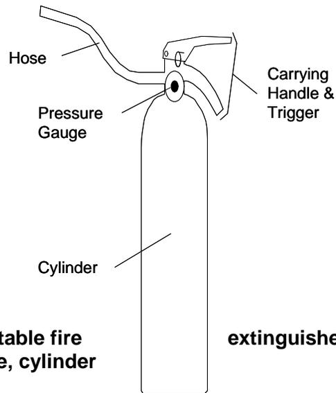
**Components of a portable fire trigger, pressure gauge, cylinder**
