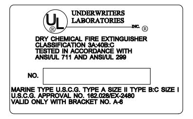
Sample manufacturer's label for a fire extinguisher, showing the Underwriters Laboratories symbol at the top, the type and classification of fire extinguisher, testing procedures used, and serial number. At the bottom of the label is marine information, including the U.S. Coast Guard approval number.
