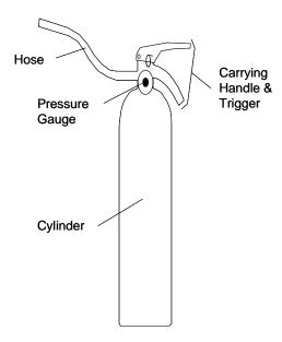
Components of a portable fire extinguisher: Hose, carrying handle and trigger, pressure gauge, cylinder
