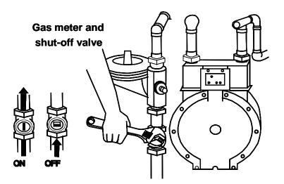
The gas meter shutoff diagram indicates the shutoff valve location on the pipe that comes out of the ground. To turn off the valve, use a non-sparking wrench to turn the valve clockwise one-quarter turn. Remember that, in all cases, natural gas flow should only be turned on by a licensed technician.
