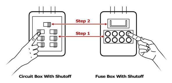
Circuit box showing shutoff steps. Step 1: Shut off individual breakers. Step 2: Shut off main breaker. Fuse box showing shutoff steps. Step 1: Pull out individual fuses. Step 2: Pull out main fuse.
